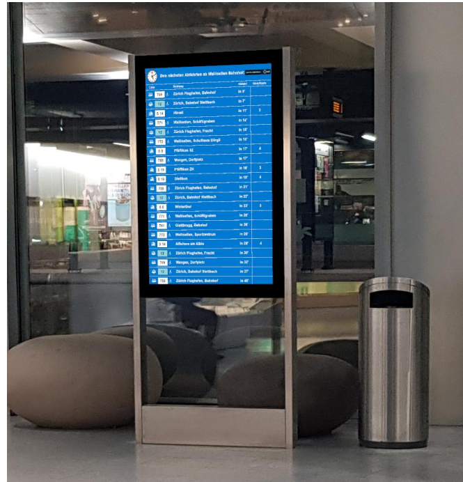
55" screen with departure times of train and bus lines
