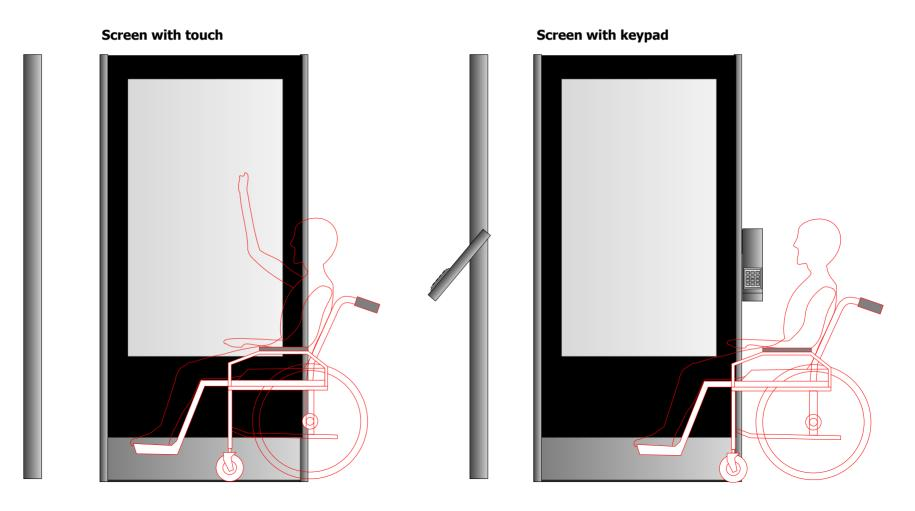
Due to the size of the screen, it is not possible for people with handicaps to touch the upper part of the screen, but it is very uncomfortable for people without handicaps to operate the lower part. Furthermore, with a touch screen you have to move away from the screen a little bit to keep an overview. The keyboard can be positioned a bit away from the screen.
